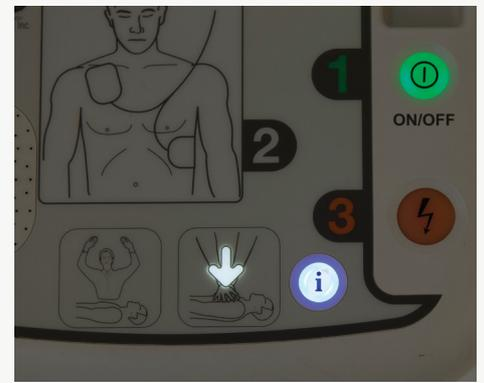
**If a shock has been delivered**, the i button will flash blue and can be pressed for CPR voice prompt.
